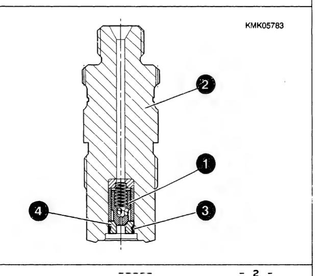
On standard in-line pumps the delivery valve separates the actual pump chamber from the injection tubing.
